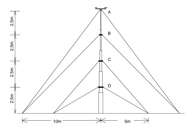
The 10m retractable mast consists of 5 sections of 2.2m aluminium tube, each section reducing in diameter so that it fits neatly into the section below when retracted. The diameter of the lowest section is 50mm, the upper section 25mm.
